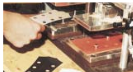
Guitar assembly – Lexan® face plate is silk screened and then laminated to mahogany or other decorative wood with precisely die-cut 3M Thermo-Bond Film.
