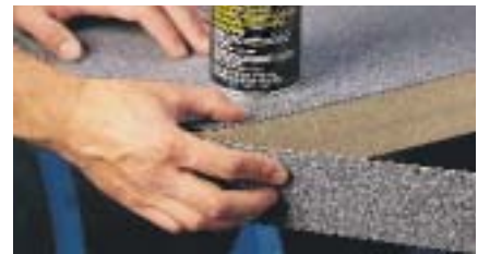
Edge banding – 3M™ Hi-Strength 90 Spray Adhesive typically bonds in 60 seconds compared to 15-20 minutes for many typical bulk contact adhesives. Strength increases to an ultimate 230 psi in shear and 25 piw in peel.
