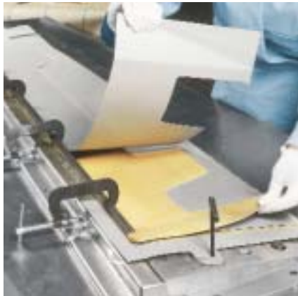
Precise fit – Available in various thicknesses and widths, 3M™ Scotch-Weld™ Film Adhesive can be die-cut into shapes to facilitate bonding of complex parts.
